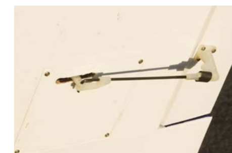
ABOVE: Retract doors are held onto legs with clamps. BELOW: Short and direct linkages to ailerons.
