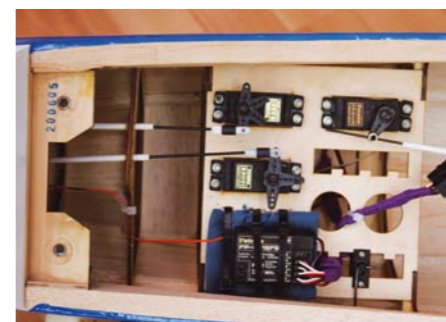
ABOVE LEFT: Retract servo has 190 degree travel with clamp connectors to aid set-up.
