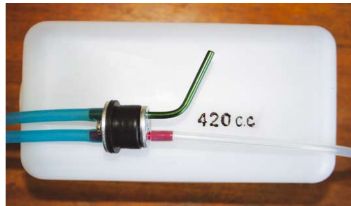
LEFT: 420 c.c. tank has colour-coded vent and feed lines.
