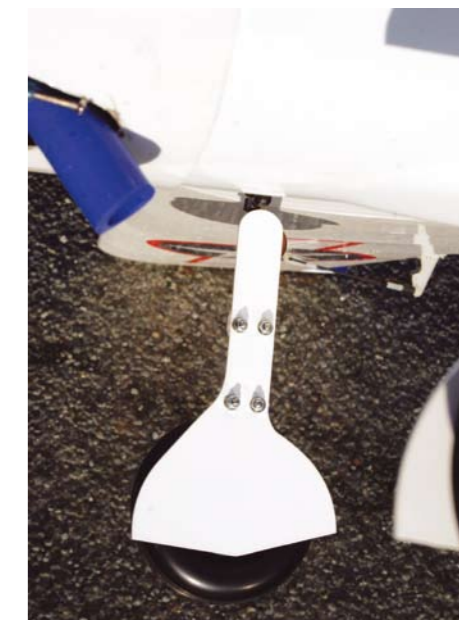
ABOVE: Retract doors are held onto legs with clamps. BELOW: Short and direct linkages to ailerons.
