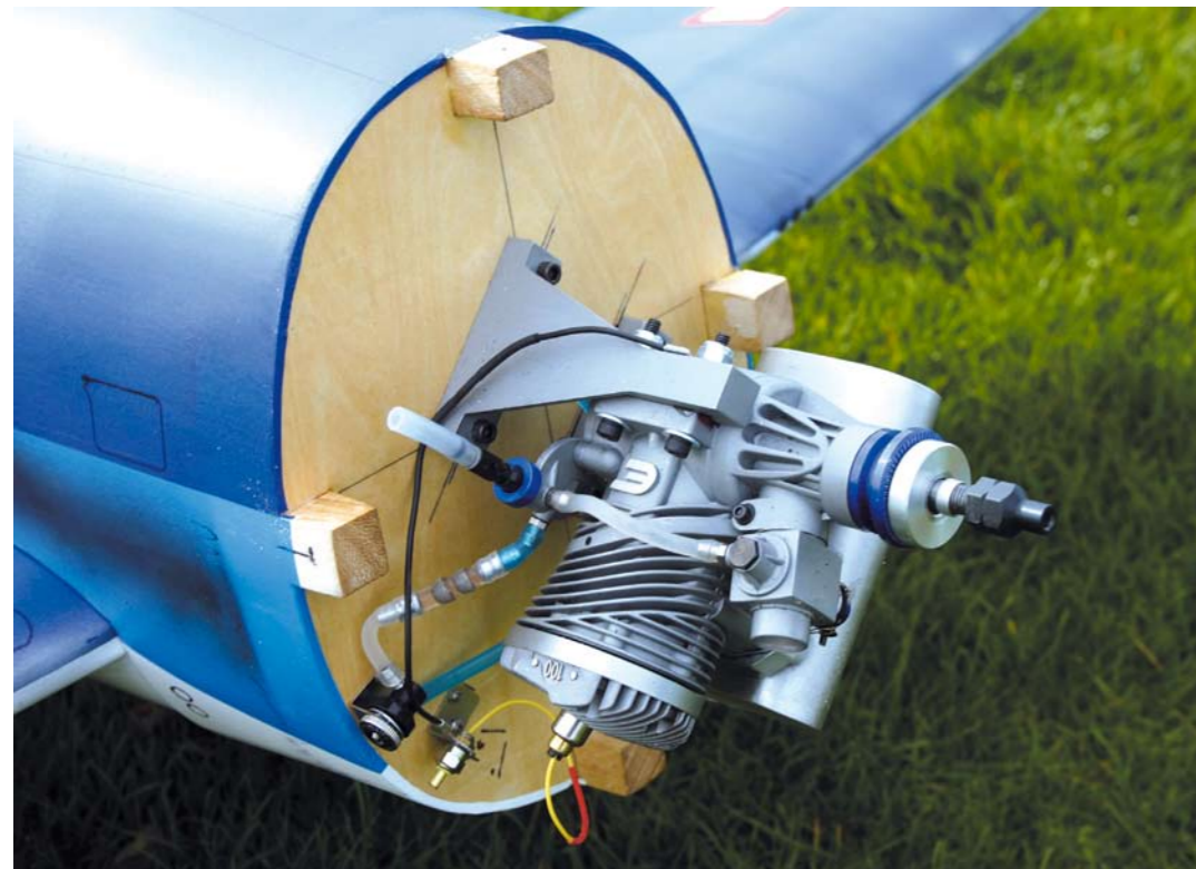
Under the cowl showing the Evo 100NX engine installation, remote glow and refueller
