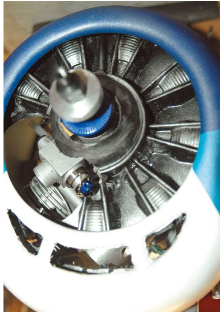
Dummy engine cut away to give clearance for carb, also gives ample cooling air inlet
