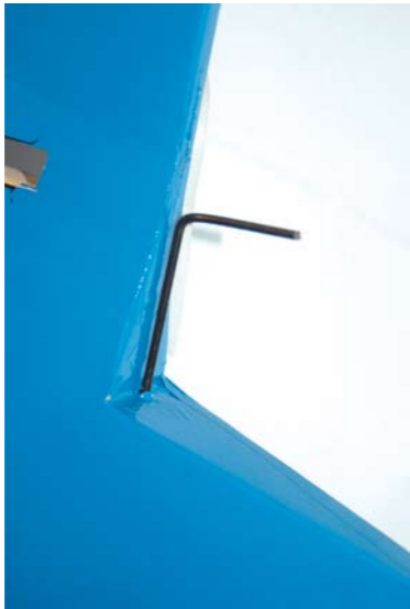
Tail wheel torque rod has to be bent in-situ
