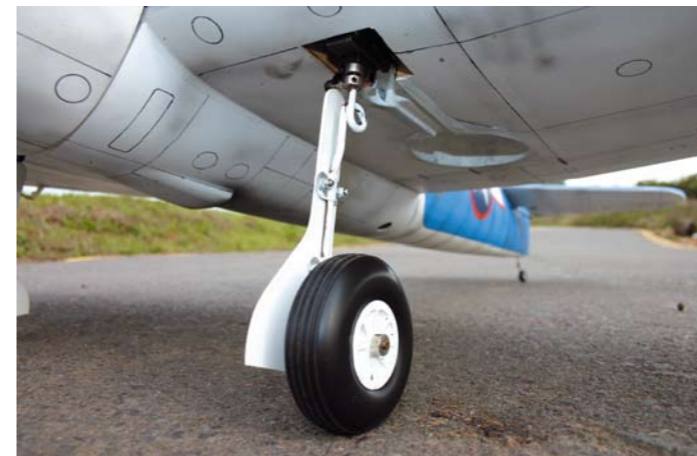
Scale rearward-retracting and rotating undercarriage
