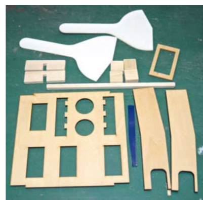
Wooden parts; radio tray, wing joiners, retract mounts radio mast (not fitted) and undercarriage fairings (I never did find out what the length of square balsa was for!)
