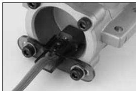
Bracket adjusted for 90-size engine
